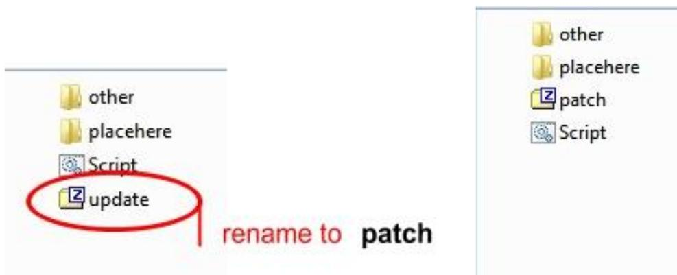
Replace in the factory firmware original "patch" by modded !
